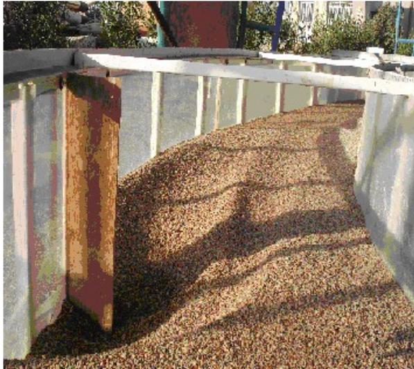
**Fig. 2. Scoring and sedimentation in Spur dike downstream**
